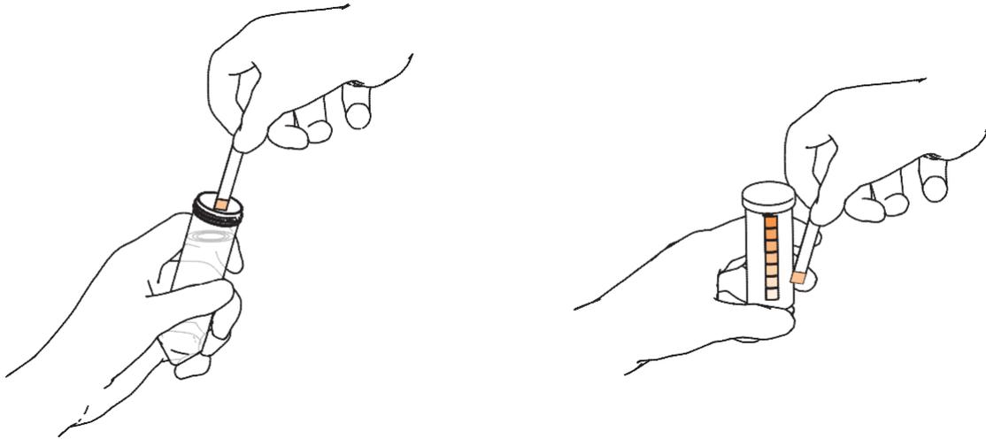
7. If the color of the reaction zone shows H<sub>2</sub>O<sub>2</sub> concentrations less than 100 mg/l H<sub>2</sub>O<sub>2</sub> perform the following steps to add an additional volume of H<sub>2</sub>O<sub>2</sub>:
